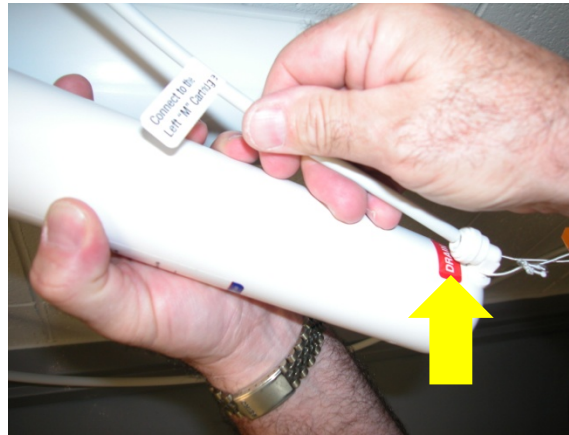
Install reject line Left & Right
